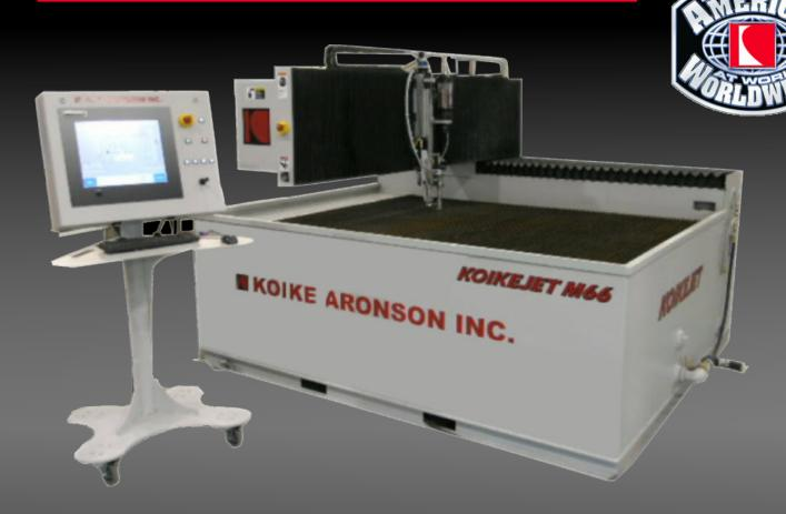
The KOIKEJET cutting system combines Koike Aronson's experience and unsurpassed customer support with the latest in waterjet technologies. Laser alignment, initial height sensing, and adjustable water level control improve cutting efficiency. Precision ground ball screw drives ensures accurate cutting motion. And the KMT intensifier pumps delivers state-of-the-art performance.
